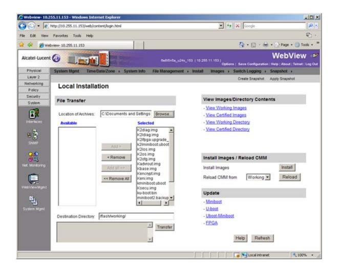
Click on the Remove All button to move all of the files to the "Available" area, then select the ku-boot.bin file and the k2Iminiboot.uboot file and click the Add button to move them to the "Selected" area as shown below.
